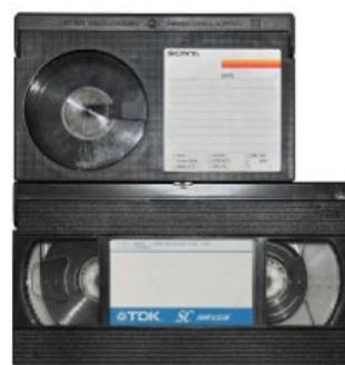
Sony Betamax tape cassette vs. a VHS format cassette
